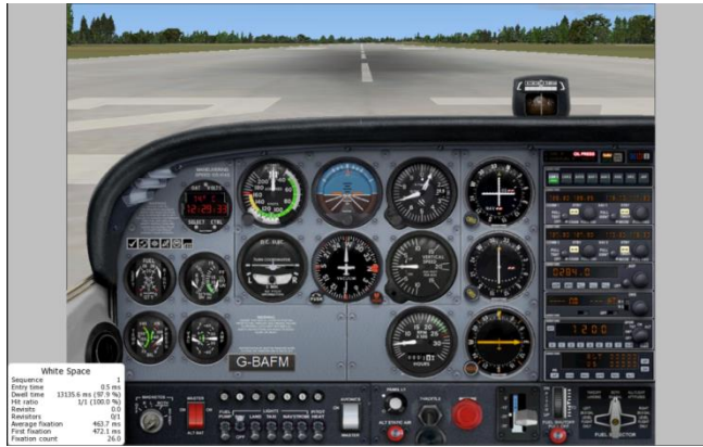
Fig. 3.5. The Key performance option displays, among others, information such as: number of fixations, duration of projection, time the first fixation occurred
