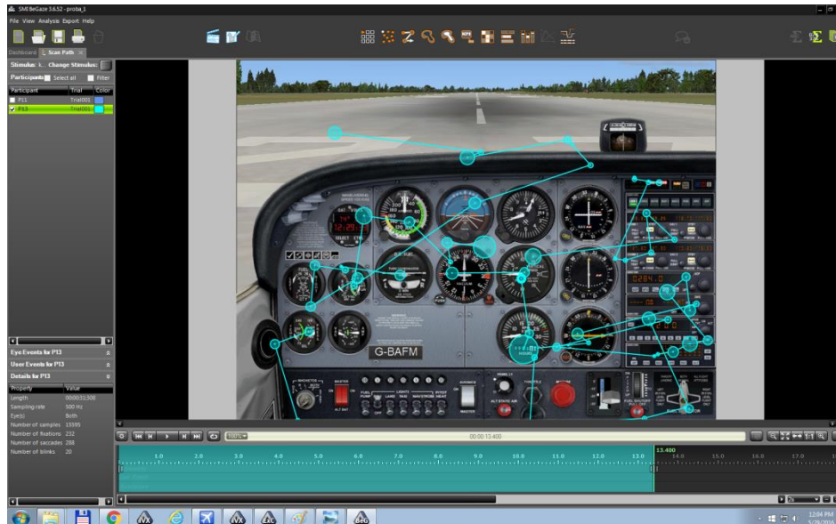
Fig. 4.2. Distribution of fixations and saccades for a person classified as a NON - PILOT , the option SCAN- PATH
