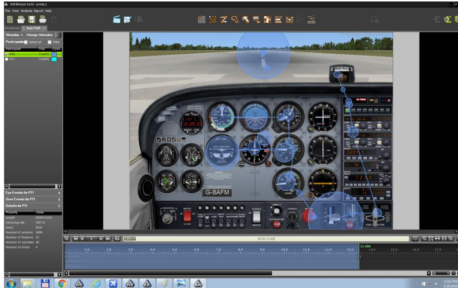
Fig. 4.3. Distribution of fixations and saccades for a person classified as a PILOT, the SCAN-PATH option
