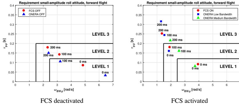
Fig. 13: Bandwidth and Phase Delay Comparison with [26].
