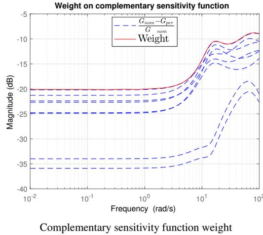
Fig. 11: Weights on sensitivity functions for regulator synthesis.
