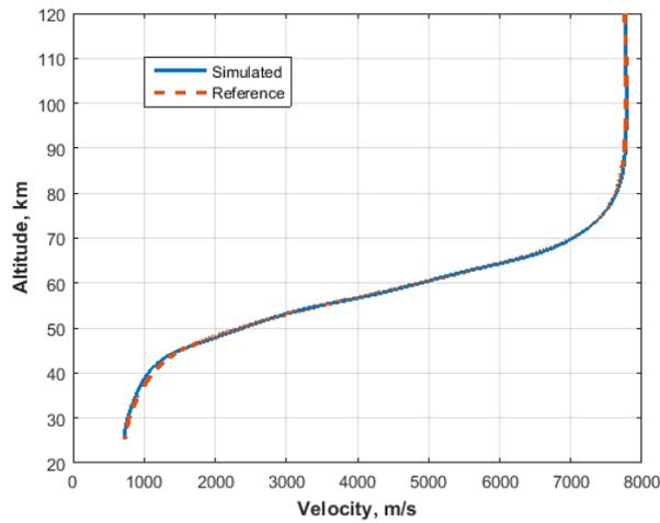
**Fig. 5** Altitude-Velocity profile using cubic spline method
