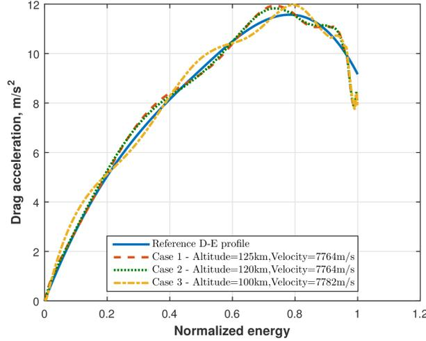
**Fig. 8** D-E profiles with same reference trajectory and different initial drag (Cubic spline method)
